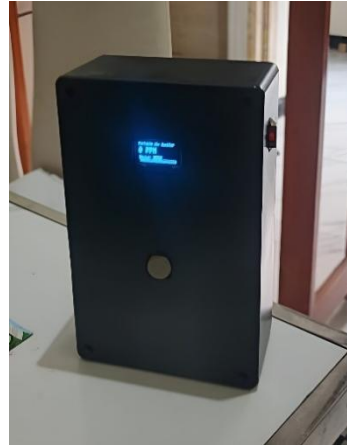
Figure 4: Actual Appearance of a Portable Air Quality Monitoring System During Indoor Testing
