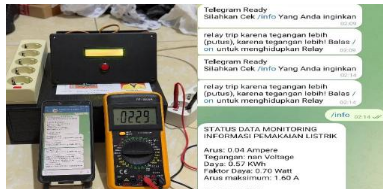
Figure 4. Result Overvoltage Testing
