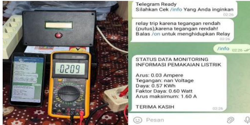
Figure 5. Result Undervoltage testing
