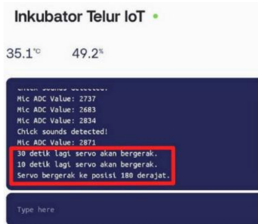
Figure 8. Blynk Notification Monitoring Servo Motor Movement in Mobile Phone
